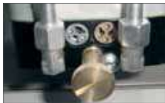
By pass valves and manual release
